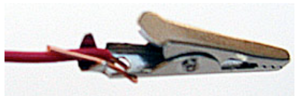
Figure 7b Bend bare end back and upward, between tabs.
